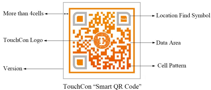
Features: Model 1 is the original QR Code. The largest version of this code is 14(73x73 modules), which is capable of storing up to 1,167 digits. Model 2 is an improvement on Model 1. The largest version is 40 (177x177 modules), which is capable of storing up to 7,089 digits. Today, the term QR Code usually refers to this type.
