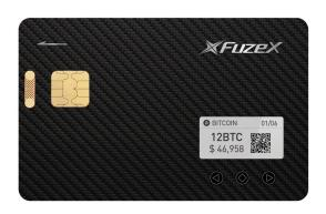
The FuzeX Card will include all the features of the Fuze Card with the additional benefit of multi-cryptocurrency integration. The FuzeX Card is identical in size and thickness as a standard credit or debit card and consists of an EMV chip, E-Paper Display (EPD), three input/option buttons and a charger terminal.
